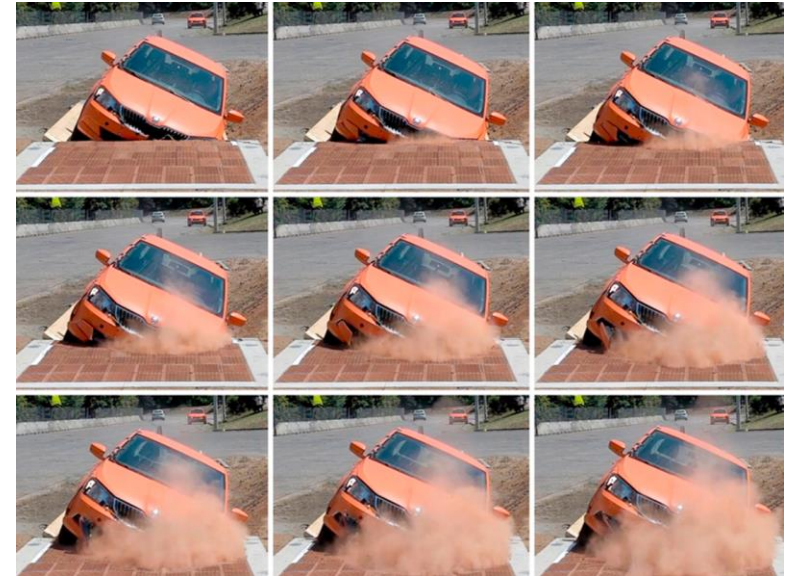
Collision of Skoda Fabia vehicle with deformable ceramic blocks
