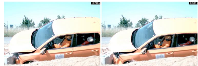
Collision of Skoda Fabia vehicle with deformable ceramic blocks
